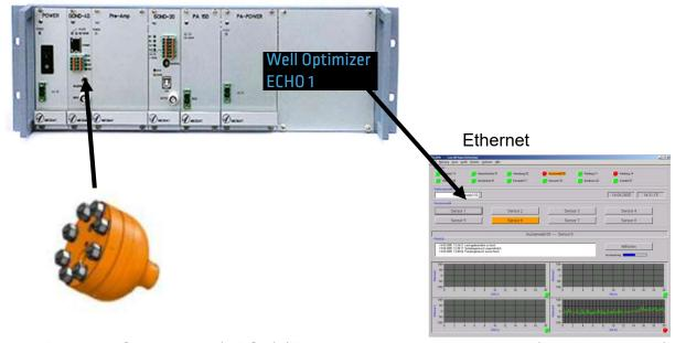
High Pressure Sensor Unit (HPSU) /Transducer measuring adapter (borehole sound)
